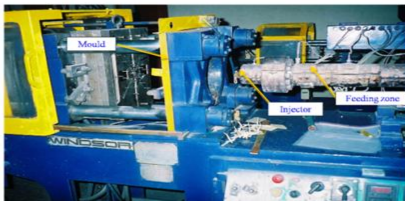
Figure 2: Injection moulding machine (GLS Polymers, Bangalore, India)
